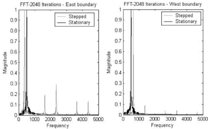
Figure 12. Fourier transform performed at the west and east boundaries of TLM Doppler simulation, implementing stepped boundary placement scheme.
