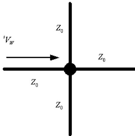
Figure 3. 2D TLM node illustrating incident pulse on West transmission line.
