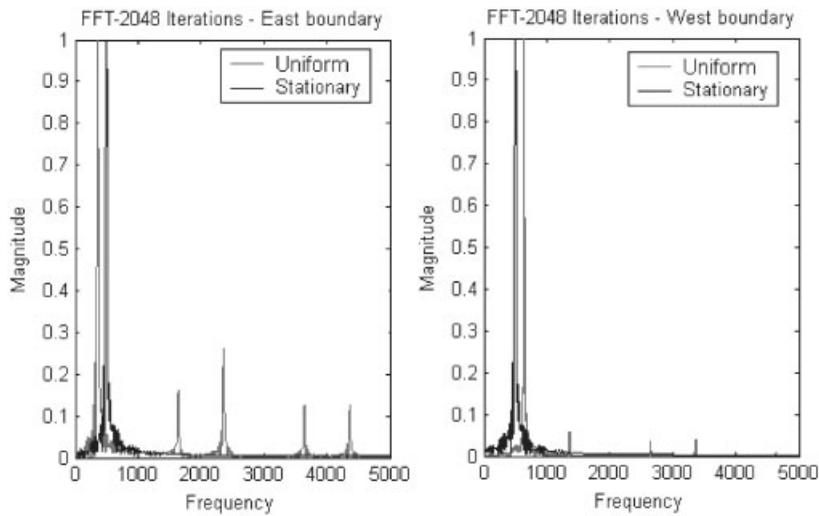
Figure 14. Fourier transform performed at the west and east boundaries of TLM Doppler simulation, implementing impedance transformation of Section 2.2.
