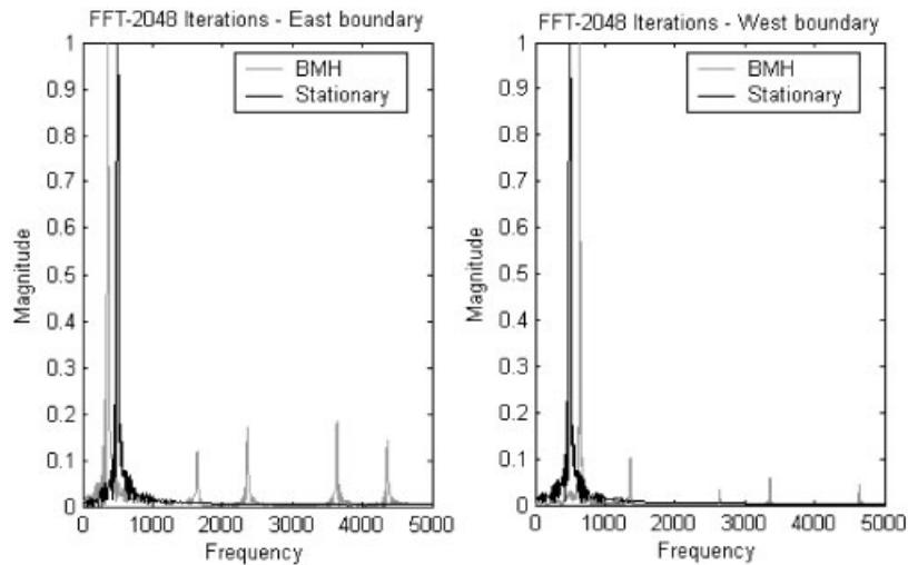
Figure 13. Fourier transform performed at the west and east boundaries of TLM Doppler simulation, implementing BMH boundary placement scheme.
