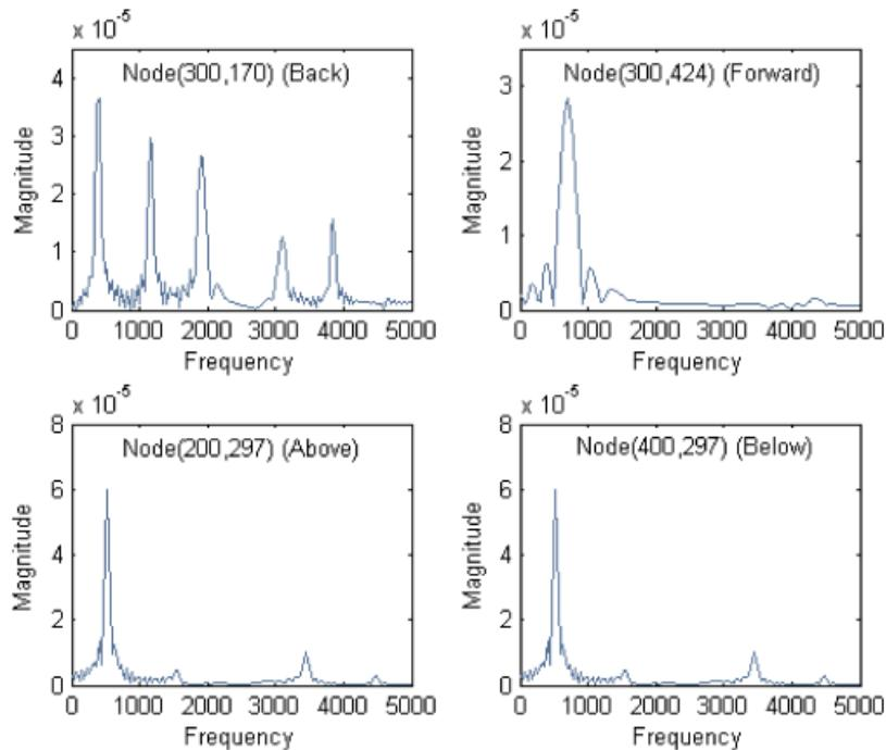
Figure 9. Fourier transform about moving source implementing O'Connor placement method, illustrating frequencies observed at stationary locations, node locations are given as  $(y, x)$  with origin at top left.
