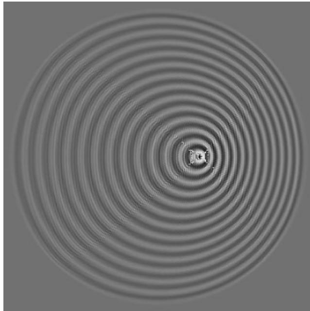
Figure 6. Sinusoidal point source, moving in the horizontal direction (east) 601 by 601 mesh resolution, source moves 1 node every 5 iterations.
