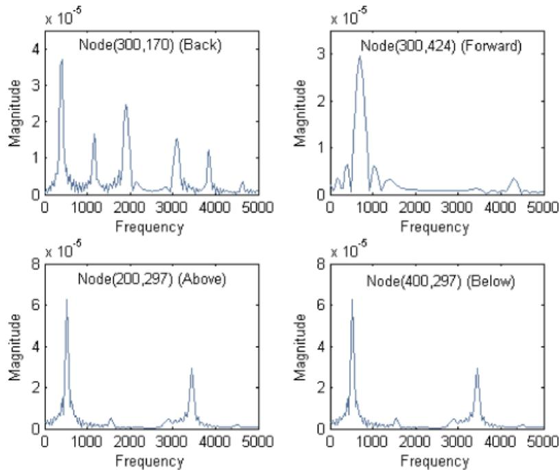
Figure 10. Fourier transform about moving source implementing impedance transformation scheme, illustrating frequencies observed at stationary locations, node locations are given as  $(y, x)$  with origin at top left.
