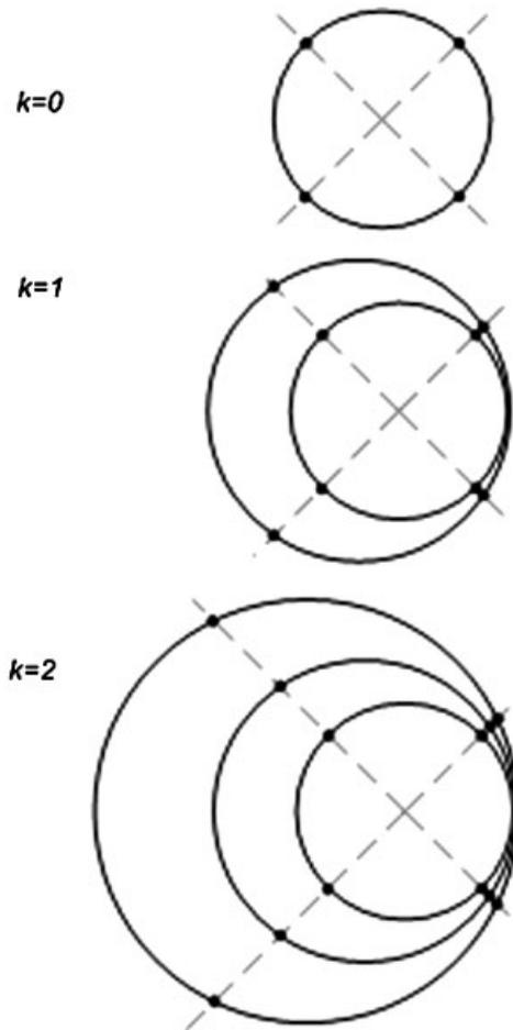
Figure 8. Illustration of moving sinusoidal point source within a rectilinear TLM mesh.
