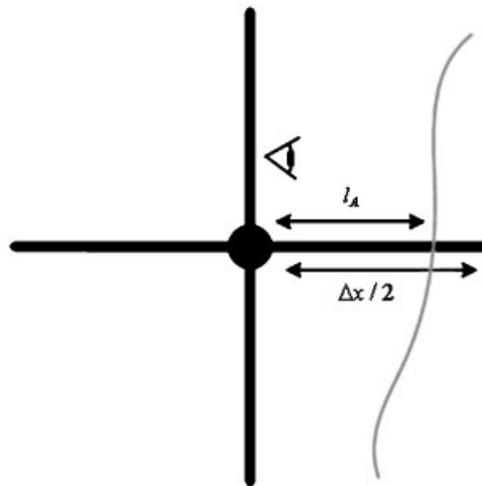
Figure 5. Illustration of scenario for impedance transformation, observer placed at node.
