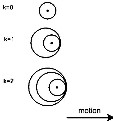
Figure 1. Illustration of acoustic emissions from a moving source.
