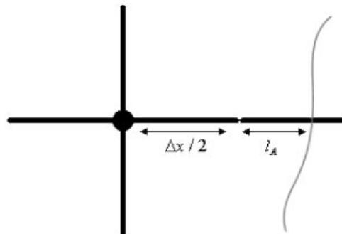
Figure 4. Arbitrary placed bounding wall after the  $\Delta x/2$  line end.
