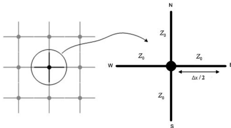
Figure 2. 2D TLM mesh and 2D scalar TLM node.
