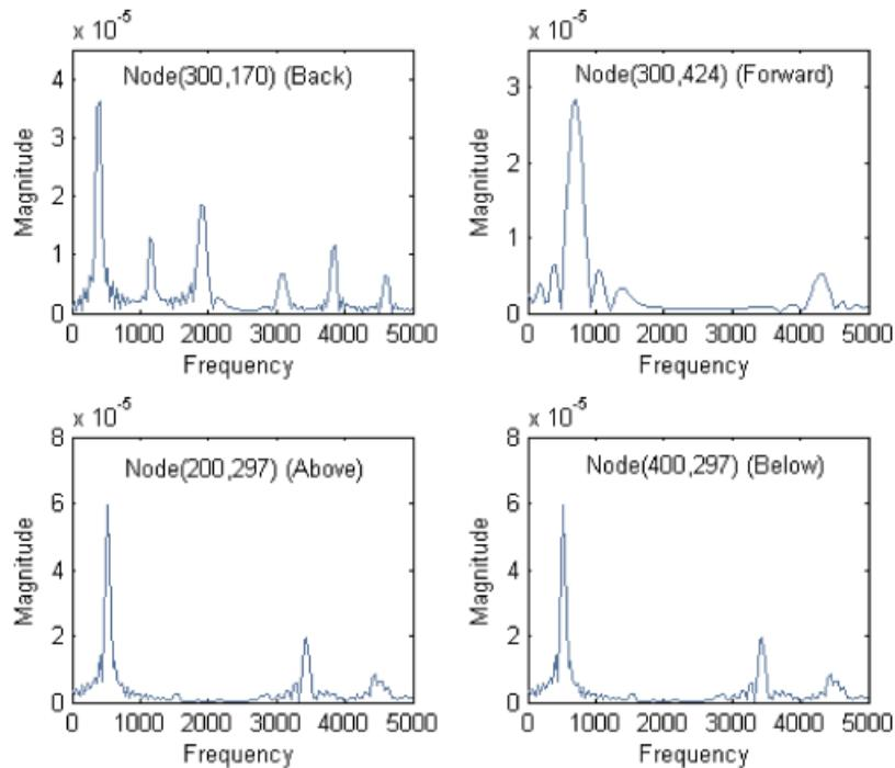
Figure 7. Fourier transform about moving source implementing stepped scheme, illustrating frequencies observed at stationary locations, node locations are given as  $(y, x)$  with origin at top left.
