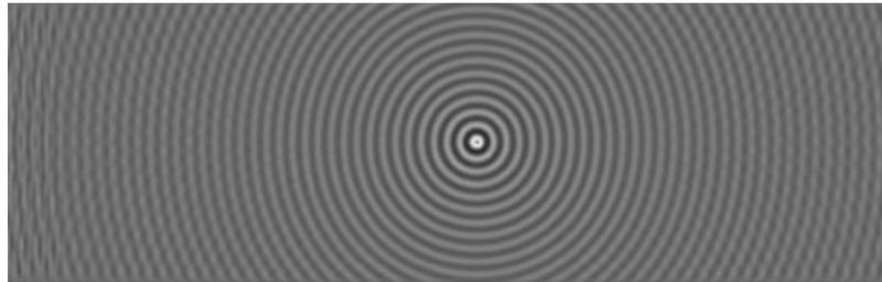
Figure 11. Doppler effect observed in TLM simulation, with moving medium (mesh), implementing stepped TLM scheme. Surface view generated using Equation (5).
