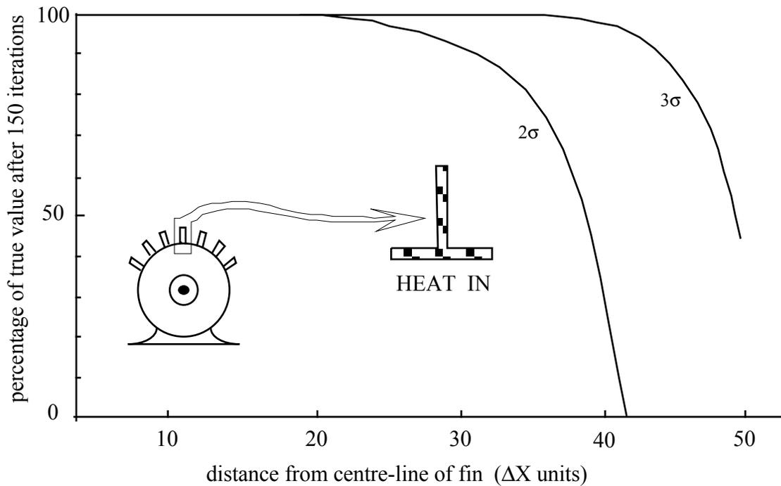
**Figure 2** Accuracy (defined as  $100 \cdot T_{\text{truncated}}(x) / T_{\text{true}}(x)$ ) as a function of distance from the centre-line of the motor cooling fin after 150 iterations for  $2\sigma(k)$  and  $3\sigma(k)$  mesh expansions.
