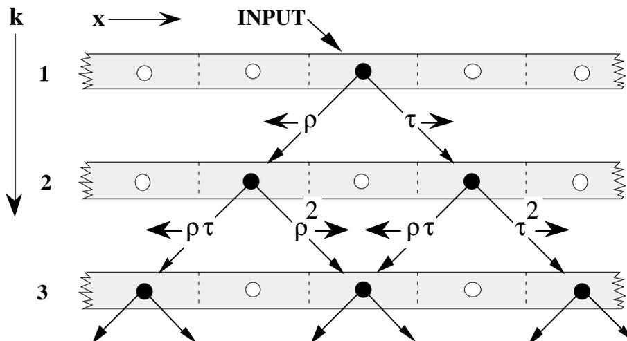
**Figure 1** One-dimensional binary scattering as a function of position and time following single-shot excitation.
