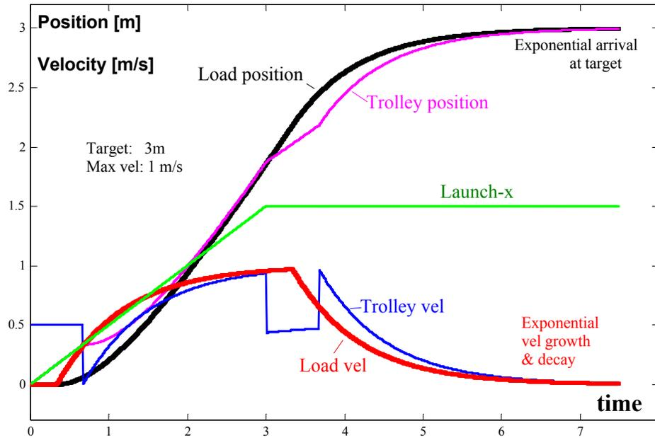
Fig.4 Simulation of a gantry crane manoeuvre, using a full TLM model.
