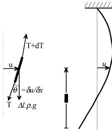
Fig.2. The forces (left) on a string element of a hanging cable under gravity, and (right) the first mode of vibration of this system.
