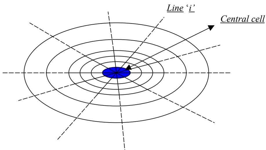
Figure 6 An orthogonal polar mesh
