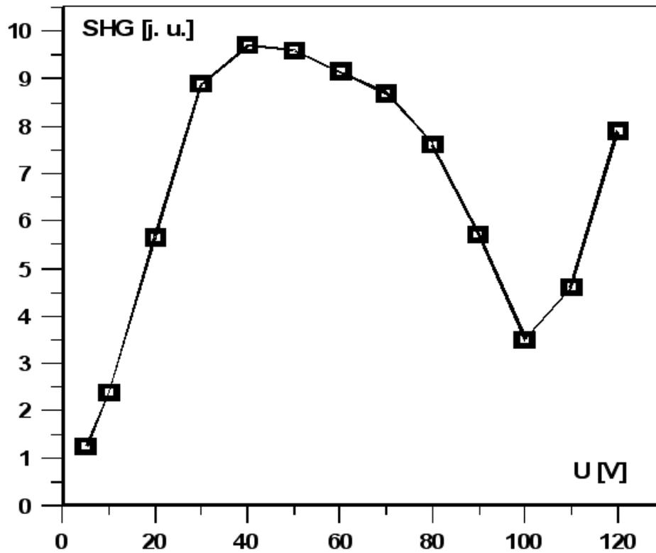
Figure 5. Photoinduced SHG intensity as function of polarizing voltage  $U$  at 77K.
