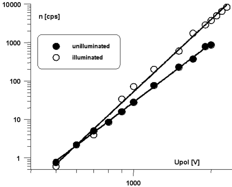
Figure 3. Logarithmic plot of count frequency as function of negative polarizing voltage.
