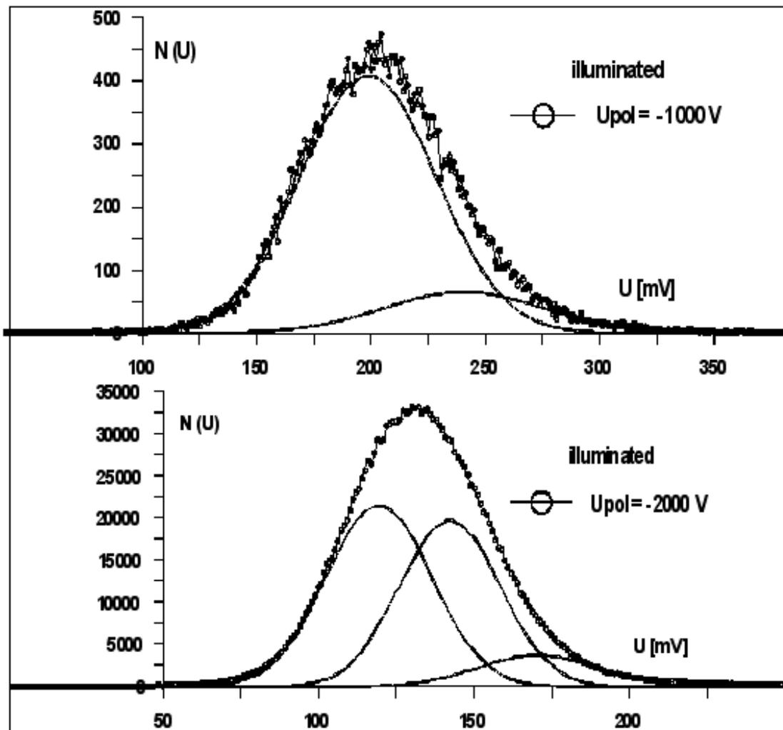
Figure 2. Exemplary pulse amplitude spectra and their decomposition into Gaussians for an illuminated sample.
