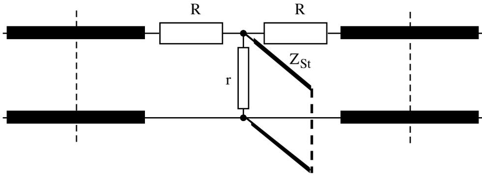
Figure 3 Lossy diffusion node with capacitive stub
