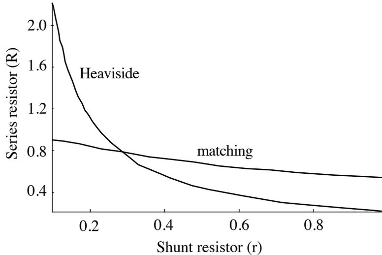
Figure 4 Plots of the matching and distortionless dependence of  $R$  as a function of  $r$  for a node with a capacitive stub  $Z_{St} = 2$ .
