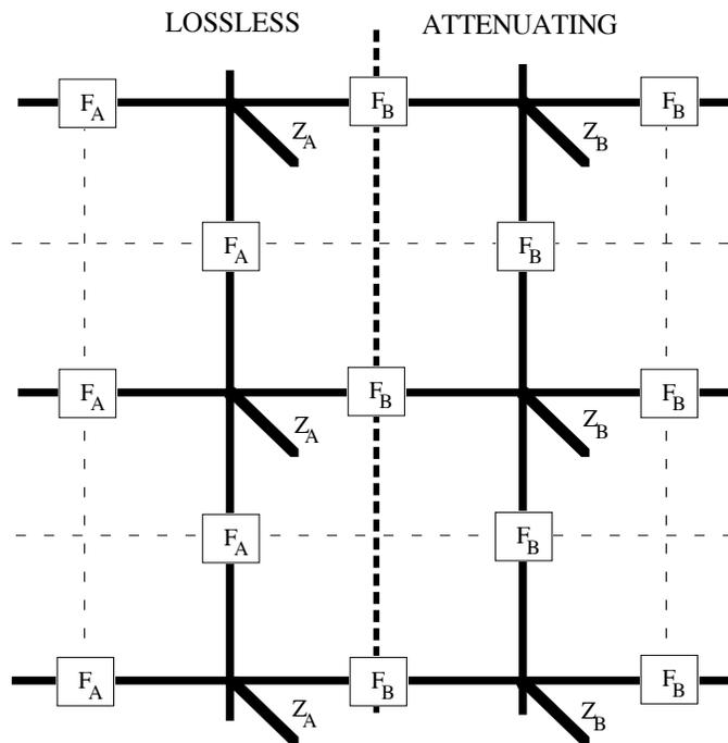
Figure 8. Fully stub-loaded mesh arranged for algorithmic simplicity. Since region A is lossless  $F_A = 1$  and  $Z_A$  is chosen so as to maintain equal loading (velocity) across the entire network. Within the attenuating region we have  $F_B < 1$  and  $Z_B$  can be set equal to infinity.
