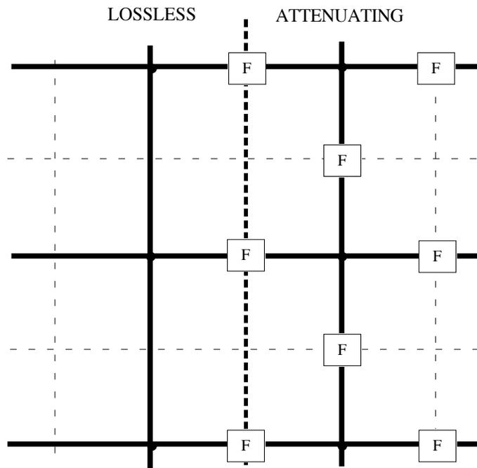
Figure 7 The interface between lossless and attenuating regions in a two-dimensional TLM network.
