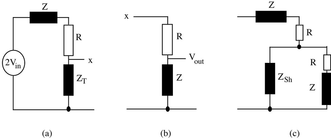
Figure 2 (a) a generalised representation of the circuit in figure 1. (b) the Thévenin equivalent circuit
