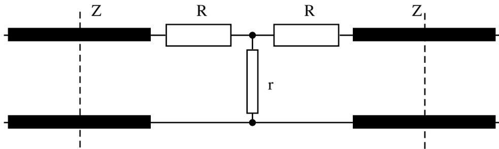
Figure 1 A diffusion node with a shunt loss
