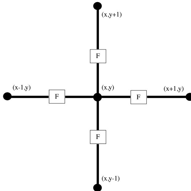
Figure 6 The arrangement of attenuating networks (designated 'F') at the centre of the lines linking adjacent two-dimensional nodes.
