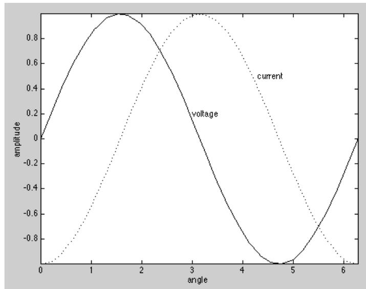
Figure 3.3 phase-lag between AC voltage and current in an inductor
