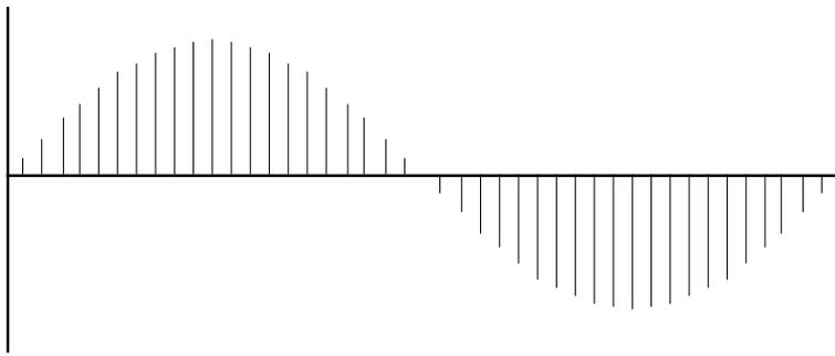
Figure 3.6 A discrete sinusoid constructed from a time series of impulses
