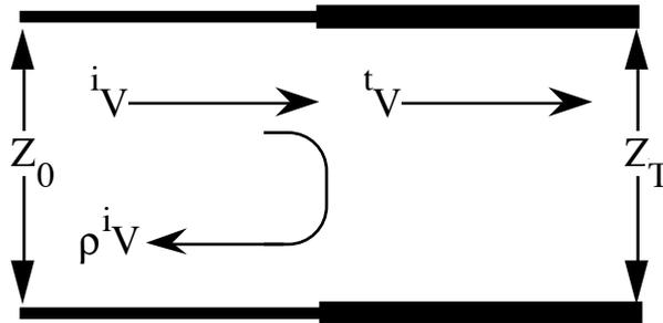
Figure 3.9 Voltage scattering at an impedance discontinuity
