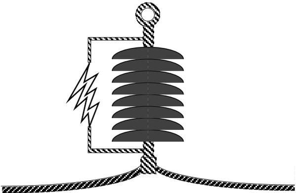
Figure 3.2 Insulator necklace on a high voltage (on-pylon) support showing a flash-over.
