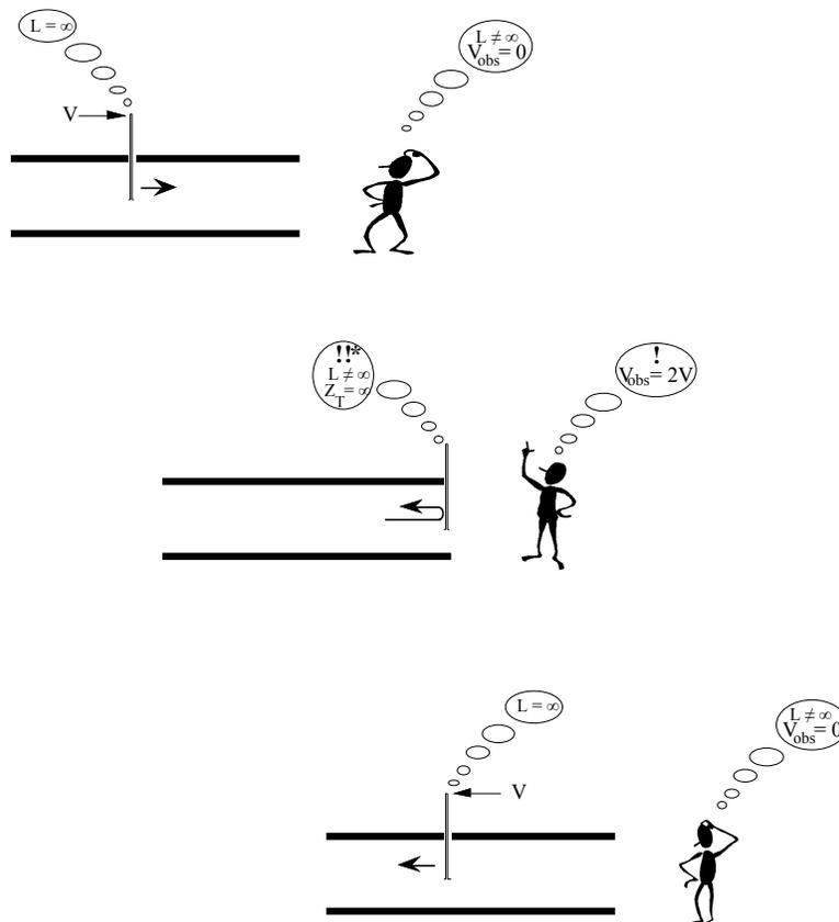
Figure 3.4 Time-history of an impulse travelling on a transmission line from two points of observation
