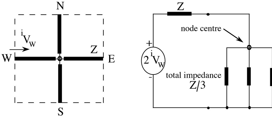
Figure 3.10 Lossless TLM node and its Thévenin equivalent
