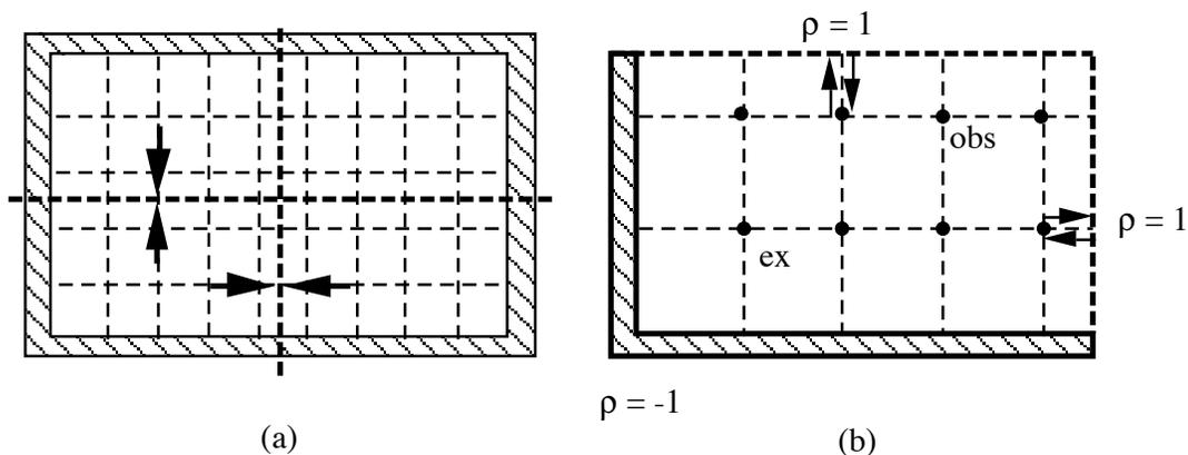
Figure 3.11 (a) A section of discretised electromagnetic waveguide showing the passage of impulses (arrows) across the two orthogonal symmetry axes. (b) Symmetry-reduced model. ('ex' is the point at which excitation signals are inserted into the mesh, 'obs' is the observation point where data is collected for subsequent use in Fourier analysis).
