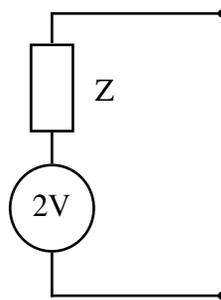
Figure 3.5 Equivalent circuit of a transmission line at the moment of arrival of a signal.
