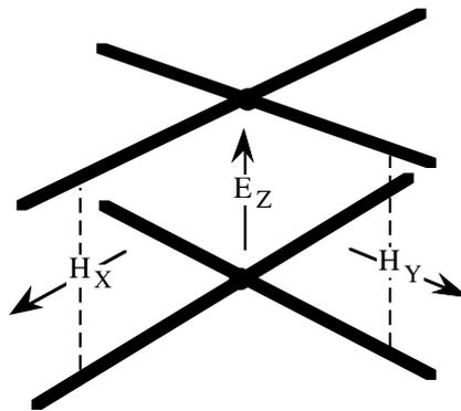
Figure 3.7 intersecting pair of two-wire transmission lines
