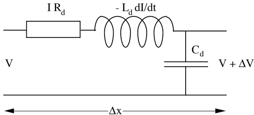
Figure 3.8 A simple LRC circuit
