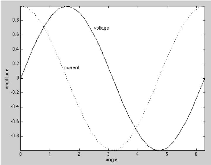
Figure 3.1 phase-lag between AC voltage and current in a capacitor
